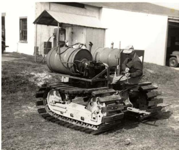
This Oliver OC3 Crawler Tractor was converted from farm use by removing the bulldozer blades and installing tanks and a spray pump in order to disperse waste oil for larviciding in the salt marsh. Oak boards were bolted onto the tracks to help keep it from sinking.
